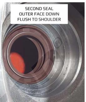
Install the second seal, oriented face-to face with the first - **DO NOT** press seal in too deep. Press the seal until the edge of the seal is flush with the housing. This ensures the weep hole is exposed, allowing any leakage to drain off, and prevent mixing gearbox oil and diff oil.
