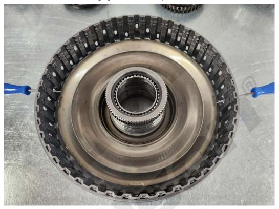
Inspect the large piston seal for any damage.
