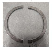
Remove the large piston retainer and the large piston return spring.
