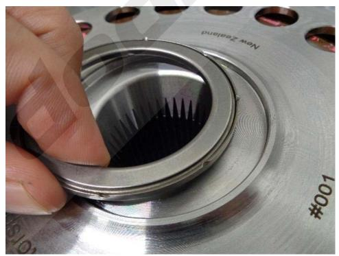
NOTE: DO NOT PLACE THE OEM SHIM/WASHER UNDER THE BEARING.
