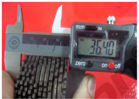
If assembling a new kit, the stack height specification is outlined below for reference.
