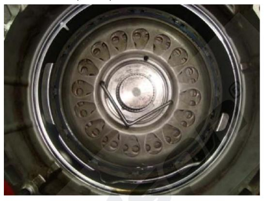
While holding the **park lever** open, spin the clutch unit anti-clockwise to loosen the lock nut. Then carefully remove the clutch from transmission.
