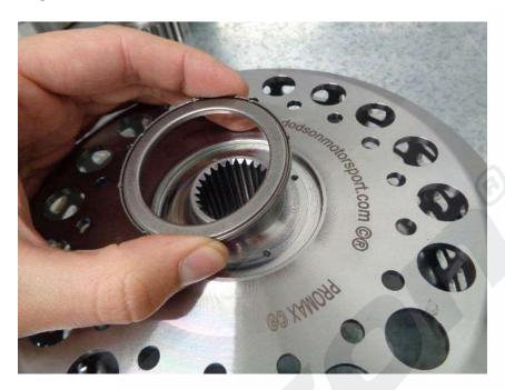
NOTE: DO NOT PLACE THE OEM SHIM/WASHER UNDER THE BEARING.
