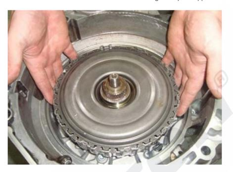
**STEP 6**Remove the oil pump drive shaft.
