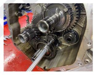
**NOTE:** Take special care when disassembling the gearbox to note the position and orientation of all the components, and to ensure that no components are misplaced.
