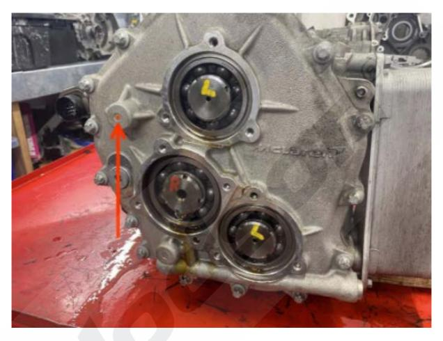
Using the included drill guide to ensure the hole is central to the sleeve, use an 8.4mm drill bit to create a hole through the end of the cover as shown.
