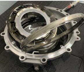
**STEP 10**Remove the circlip retaining the inner ring of the diaphragm.
