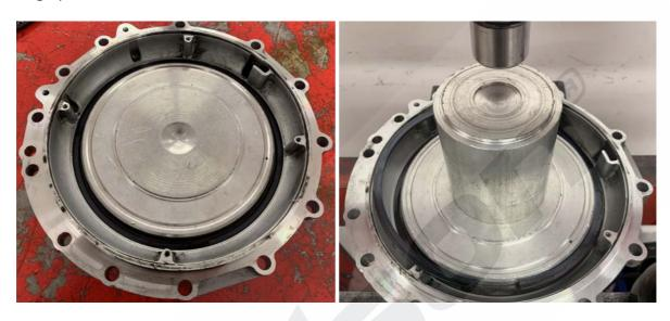
**STEP 8**Take the diff cover out of the press and remove the circlip, shim and diaphragm spring.
