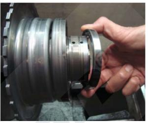
For Dodson Superstock Clutches, the machining of the clutch center is now finished.
