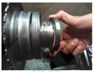
Once the bearing fits the clutch center, machining is finished.
