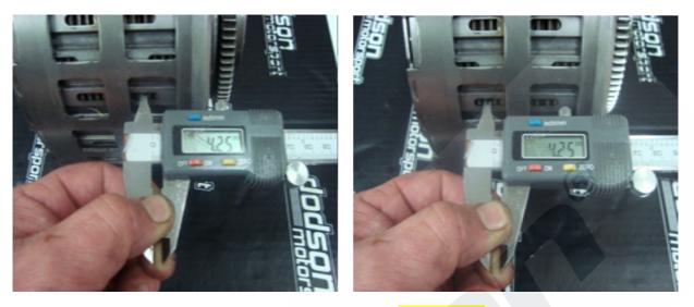
The target clearance reading for the 'A' Clutch is between 2.6+/-0.2mm
