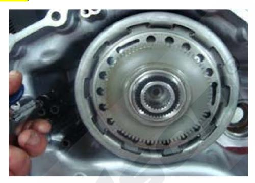
When the clutch is fitted for the final time, do not forget to fit the clutch center circlip.
