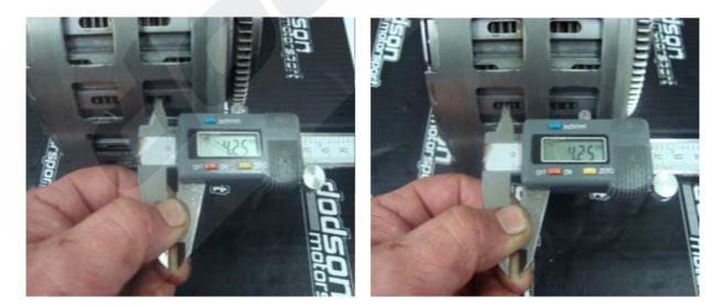
The target clearance reading for the A clutch is between 2.6mm +/- 0.2mm.
