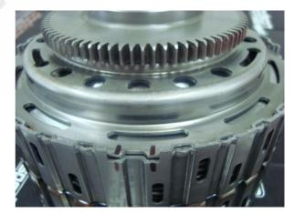
Remove the factory circlip. You can now remove the factory **A-piston** from the clutch center.
