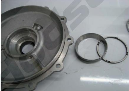
Make sure to take out the spacer below the taper roller bearing sleeve.
