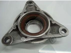
Be careful not to damage the seal during this process. It's recommended to have the pressing tool diameter around 59 mm.
