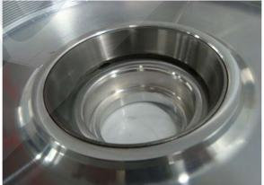
Make sure the spacer below the taper roller sleeve stops turning after installation.
