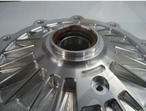
Use a pressing tool around 53 mm diameter to make sure the seal gets pressed evenly. If a smaller diameter is used then it will damage the seal.
