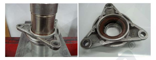
Be careful not to damage the seal during this process. It's better to have the pressing tool diameter around 59 mm.
