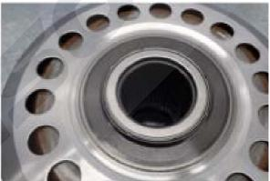
NOTE: DO NOT PLACE THE OEM SHIM/WASHER UNDER THE BEARING.
