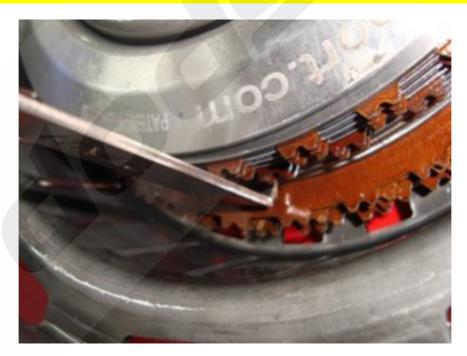
NOTE: On the large clutch, the clearance should be 2.4mm +/-0.2mm. For the 6/7 kit (DMS-8009) the clearance should be 2.6mm +/-0.2mm.
