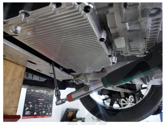
**NOTE:** A longer mounting bolt is included in the kit, to be used if the **Dodson Motorsport Filler Kit** is installed. The extra length allows for the bolt to pass through the hose clamp. If the filler kit is not installed, this bolt is not required.
