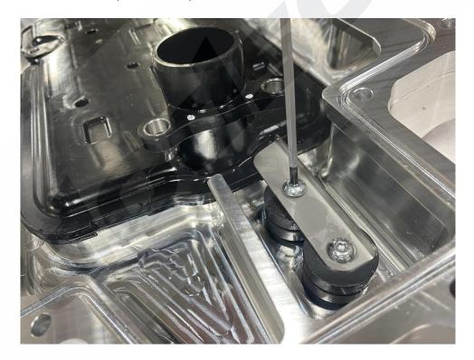
NOTE: The filter hold down plate will bend slightly as the bolts are tightened - this is normal.
