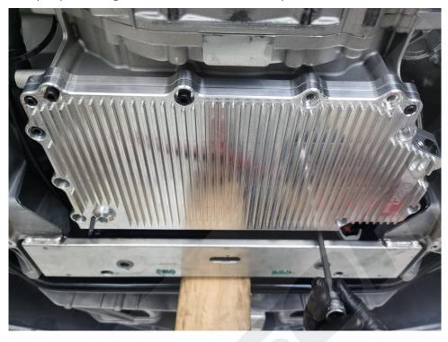
Note: A ball end hex key will be required to install and torque the four mounting bolts along the rear edge of the sump, as shown below.
