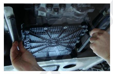
Note: for v8 applications the customer will have spacers and replacement screws for the under tray. These are required for the sump to fit.
